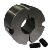
Where possible it is a good idea to use a Taper lock bush to transmit the drive. It clamps the shaft, is easily replaceable and gives flexibility on the shaft size.
